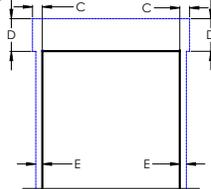
Minimum Mounting Surface Areas for Model 944      Minimum Mounting Surface Areas for Model 944WL
